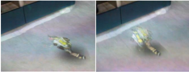
Figure 11. Calibration errors between units result in ghosting artifacts in projector overlapping regions. (left) The character in a single projector, and (right) in an overlapping region.
