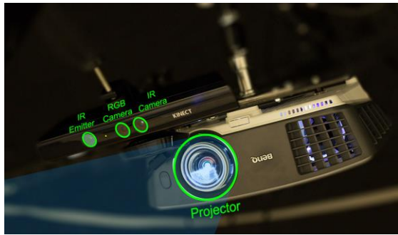
Figure 2. Each projector + depth camera unit (a procam unit) consists of a commodity wide field-of-view projector, depth camera and computer.
