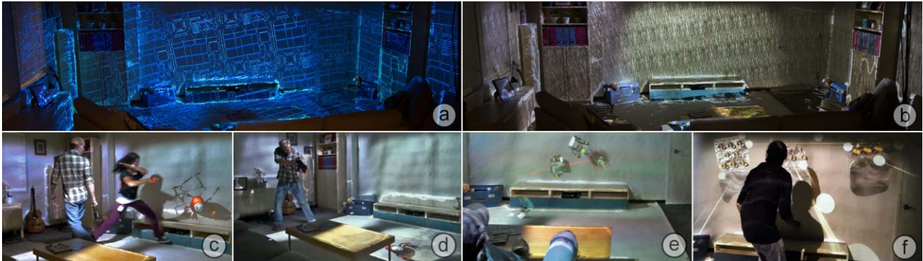
Figure 1. RoomAlive is a proof-of-concept system that transforms any room into an immersive, augmented gaming experience. E.g. RoomAlive can change the room’s appearance to be (a) Tron themed, or (b) a swampy river. In an example Whack-A-Mole game, players physically (c) whack or (d) shoot moles popping out of their floor, walls and couch. (e) Players control a robot running around the room and shoot enemy robots using a video game controller. (f) An adventure game where players avoid deadly blow dart traps with physical body movement. (All images in the paper were captured live; with the real-time working prototype).
